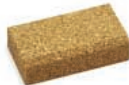
For holding glasspaper, made from compressed cork with bevelled edges. Size: 4 1/2 x 2 1/2 x 1 1/4 in.
