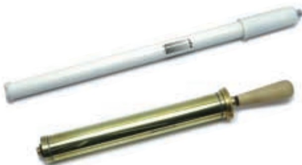
Suitable for blocking off or air testing pipes of 3½ to 6in; 89 to 150mm diameter. Tough rigid plastic central mandrel has inflatable replaceable collar secured by 2 clips. Central nipple is for connection to U Gauge. Reverse end of plug has removable stopper for an air test. Replace stopper and use as a drain plug for blanking off pipes. Equipped with Schrader valve inflation hose. Maximum inflation pressure 12psi 0.86 bar. Ideal for use with 174Z Air testing kit. Use with pump 1308Q see below
